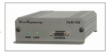
The CLR-102 is also an adapter, enabling the use of PoCL cameras with standard (non-PoCL) Camera Link frame grabbers. The CLR-102 powers the camera and incorporates the PoCL SafePower feature.
