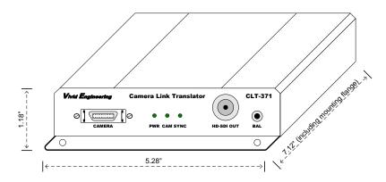
Figure 6-1: CLT-371 Cabinet Dimensions
