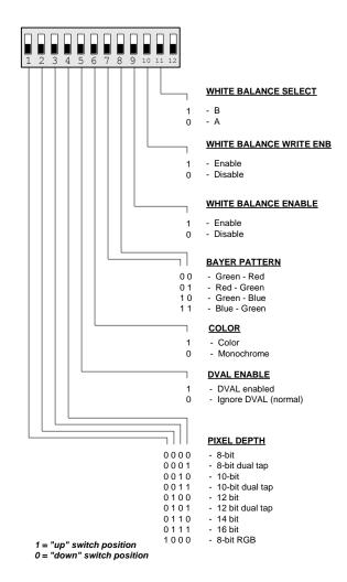
Figure 2-1: Mode 1 Switch Definition (Camera)
