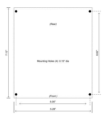
Figure 6-2: CLT-371 Mounting Footprint
