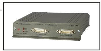
The CLR-111A supports <u>all</u> Camera Link configurations (base, medium, full) with pixel clock rates up-to 85 MHz and front-panel link status LEDs identify an active connection. The CLR-111A also supports 80-bit extended-mode applications.
