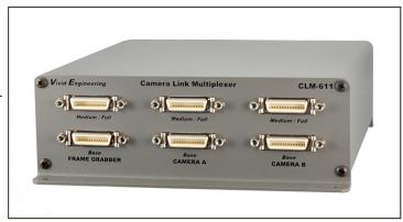
Camera Link interface signals (serial or camera control), and an external RS-232 port. An inexpensive optional adapter supports control of the CLM-611 via a PC USB port. Multiple CLM-611s may be cascaded to support more than four cameras.
