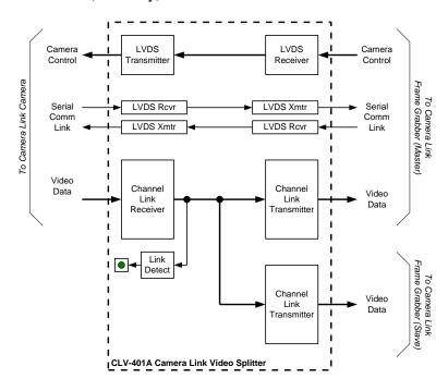
Figure 1-1: CLV-401A Block Diagram
