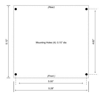
Figure 3-2: CLV-401A Mounting Footprint
